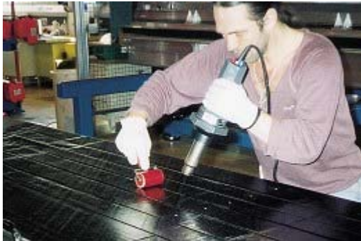
Coating a wing flap with carbon for the Airbus A 320
